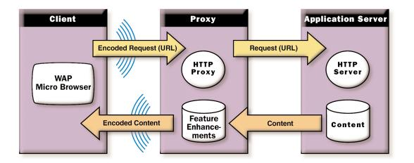
Figure 2: WAP's Optional Proxy Model Supports Network-Based Optimizations
